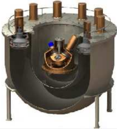
Figure 1: Computer view of the ZEPLIN I experiment showing the target vessel with three PMTs encased in an active veto system.
